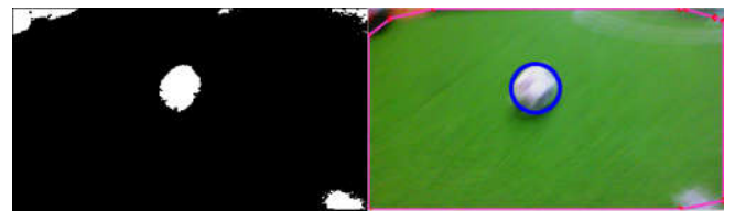
Fig. 5. Blurry image caused by low FPS when robot is walking towards the ball
