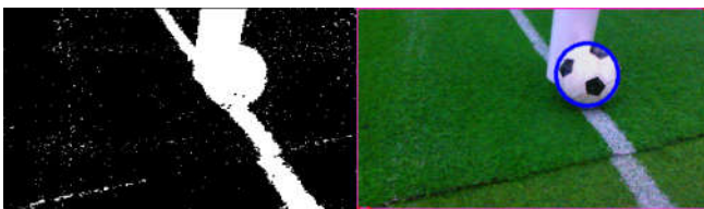
(b) White contour of ball, line and goalpost fused and ball still detected
